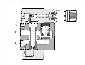
The Z\*-P type valves are used when a branch with a lower pressure than the main one is desired in the hydraulic circuits.
